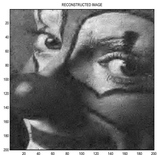
**Section 10-14.3** Denoising of clown image using 2-D db3 Daubechies wavelet transform.
