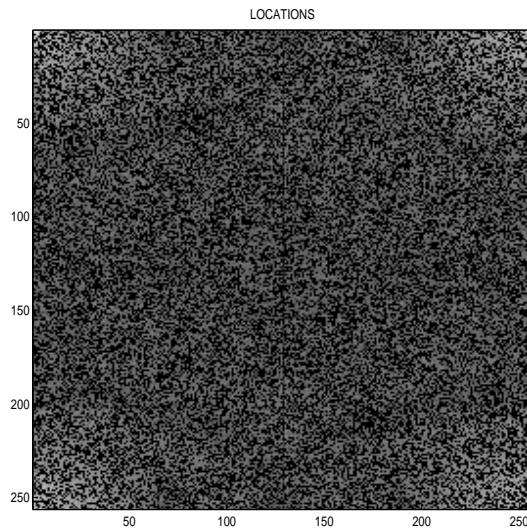
[Section 10-18.1](#) Shepp-Logan phantom reconstruction from about half of its 2-D DFT values (excluding conjugate symmetric values).
